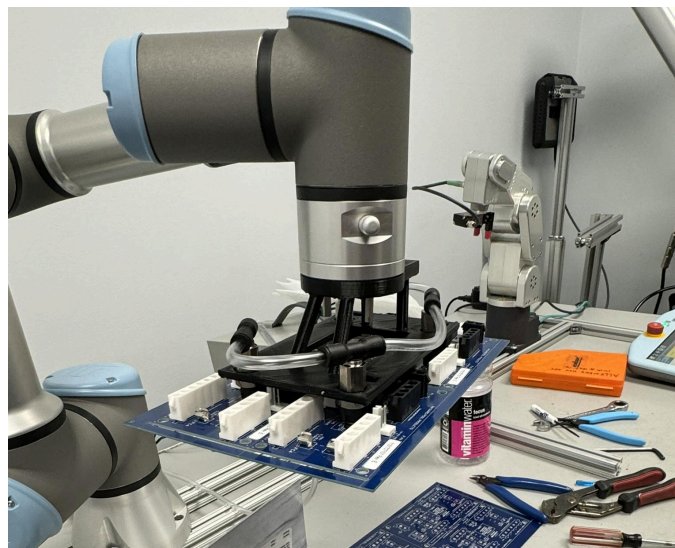
Fig. 1: PCB being picked up by UR3 Robot
